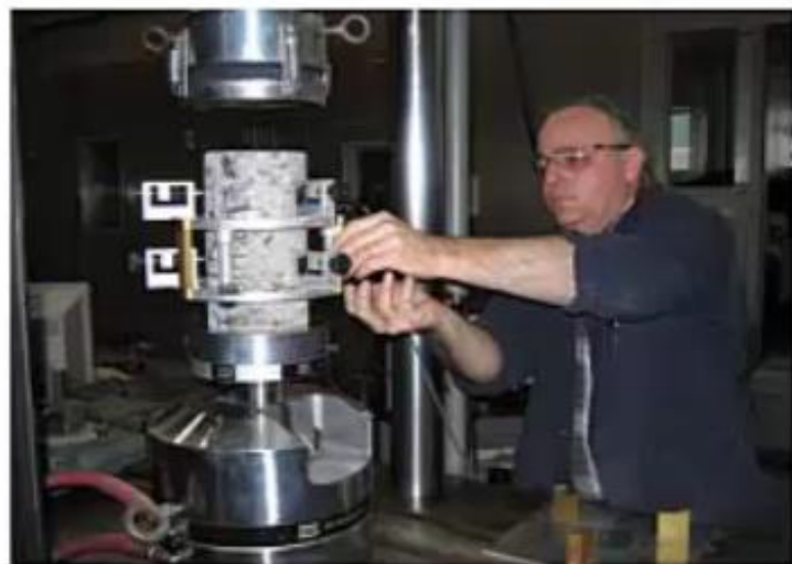
Stiffness Damage Test (SDT)
